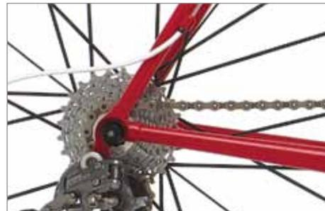
Ritchey forged socket dropouts are bombproof yet weigh a scant 17 grams a pair.
