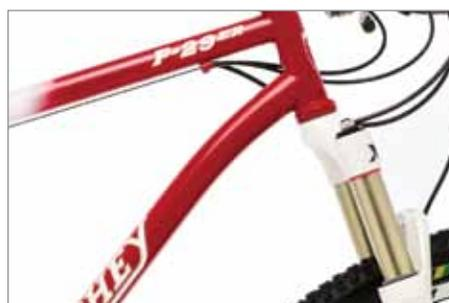
The heat-treated downtube has a bend to accommodate fork crowns.
