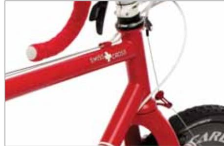
Proprietary forged, heat treated and machined integrated head tube uses standard Ritchey drop-in bearings and saves 80 grams over a standard head tube and cups. It also makes for a stronger front triangle, and more room for shouldering.
