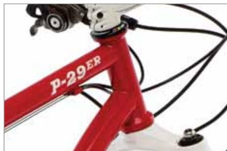
The forged and machined integrated headtube uses standard 1 1/8" steer tubes and Ritchey drop-in headset bearings, but narrows to 32mm at the thinnest section—almost the size of a 1-inch steer tube. It's a stronger design that allows for an 80 gram weight reduction over a traditional 1 1/8" steer tube design. It also makes for a stronger front triangle.
